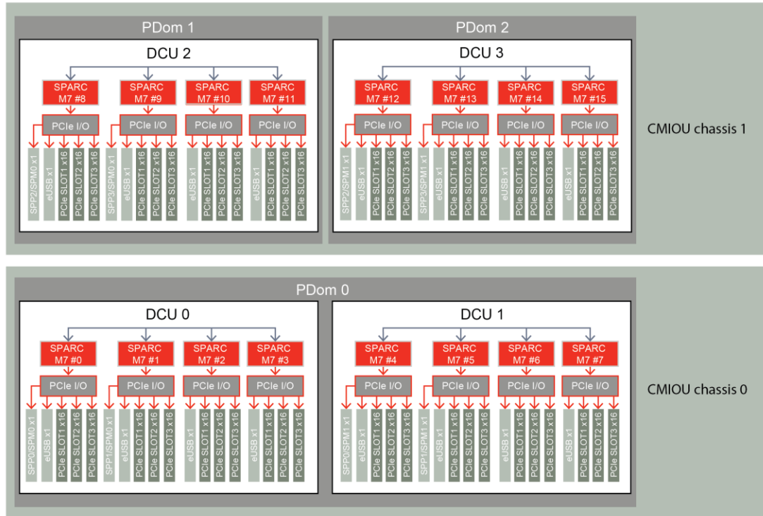
Figure 22. The SPARC M7-16 server is divided into four domain configurable units (DCUs) which can be flexibly combined to create one, two, three, or four PDom (three PDom shown).
